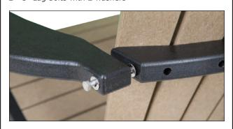
Fasten the back of the arms to the chair back using the 3" lags. Place a washer on the lag. then insert the lag into the arm. Place a second washer on the lag. Tighten the lag securely to the chair back. Be sure your lag follows the pilot hole in the back.
