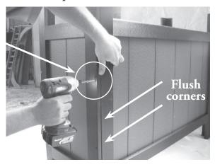
**Step #2** With the shorter overhang situated above the shelve opening, place bar top on the side uprights. Then fasten all sides using 3/4" screws.
