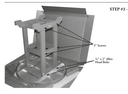
First fasten the Second Base to the Aluminum Frame of the Top using 4-1/4" x 2" Allen Head Bolts and 4-1/4" Flange Nuts. Second fasten the Footrests and Cross Support to the Base using 3" Screws.
