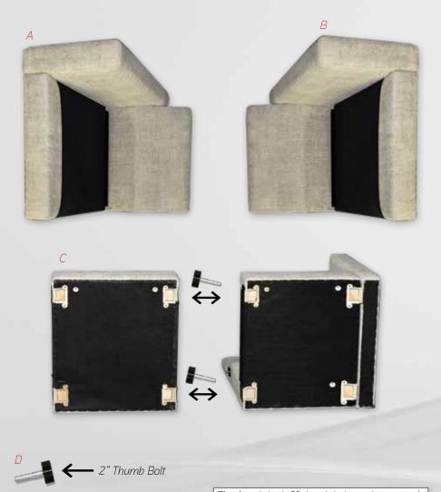
Tip: Attach both 2" thumb bolts to the seat unit first, before trying to slide the latch plate down.
